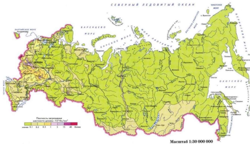
Figure 3 Map of ^{137}\text{Cs} contamination of Russia by the end of May 1986 ( \text{Ci}/\text{km}^2 ) [2]
