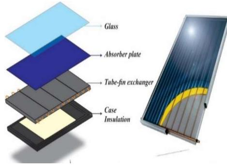
**Fig.3.** *Principal diagram of flat solar collector in parts*
