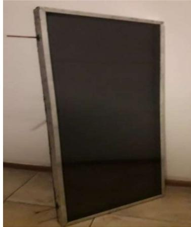
**Fig.4.** *Flat solar collector mockup*
