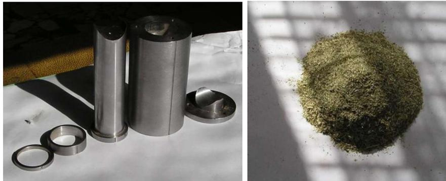
**Fig. 4.** Laboratory pressing preparation for the crushed powder of the energy crop *Amaranthus caudatus*
