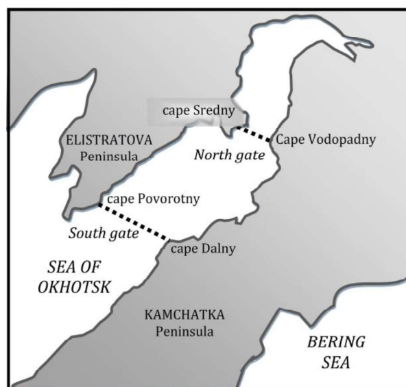
Fig. 1. Map diagram of the placement of the Northern and Southern gates of the projected Penzhinsk Tidal Power Plant [11].
