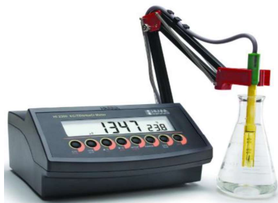
Fig. 4 - Laboratory conductometer for EC / TDS / Salinity with ATC - HI 2300. [5], [6]
