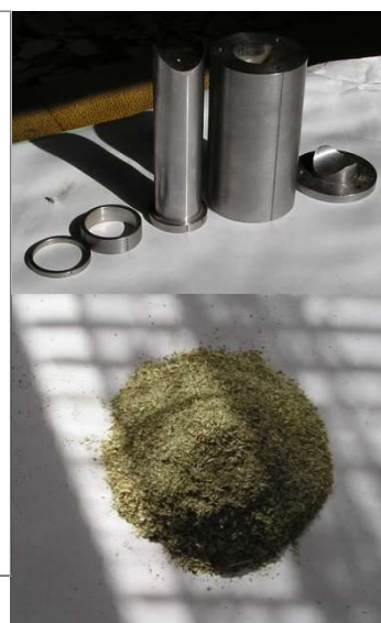
Laboratory pressing preparation for the crushed powder of the energy crop Amaranthus caudatus
