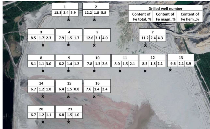
Fig. 2. Average contents of various forms of iron for wells drilled at the tailing dump
