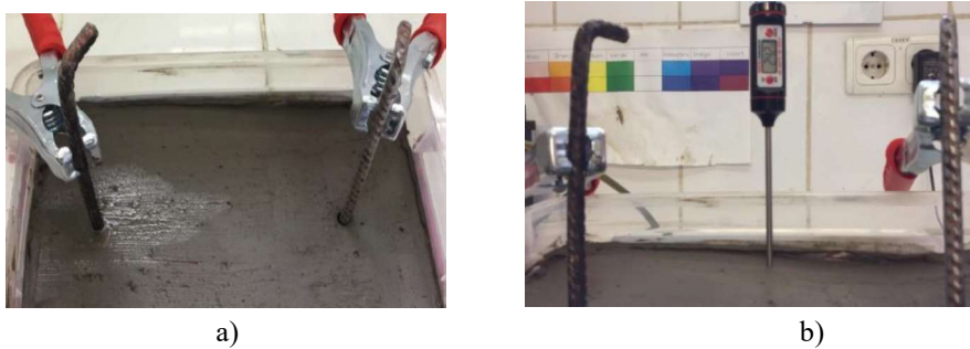
Figure 5. Experimental model: a) the film of water formed around the cathode; b) temperature measurement in the soil sample
