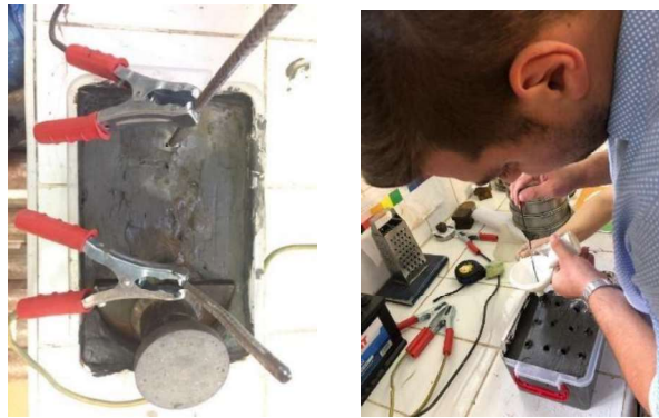
Figure 3. Experimental assembly a) for variant 2; b) for variant 3 - filling columns with lime in the experimental model
