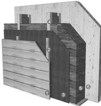
*Fig. 2 Scheme peripheral wall – CLT variant [14].*
